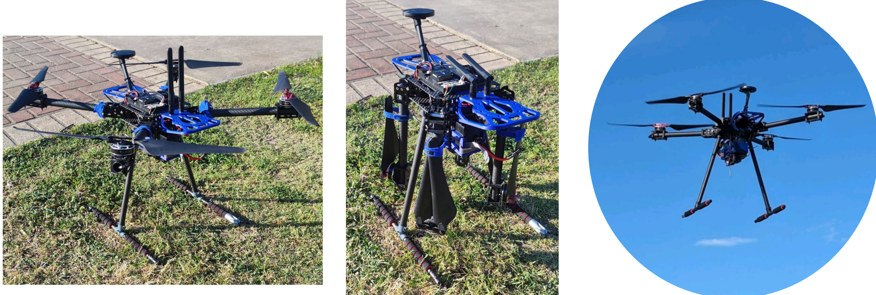
Folding 680mm quadcopter with 17 inch folding blades and a 6S 10Ah battery
